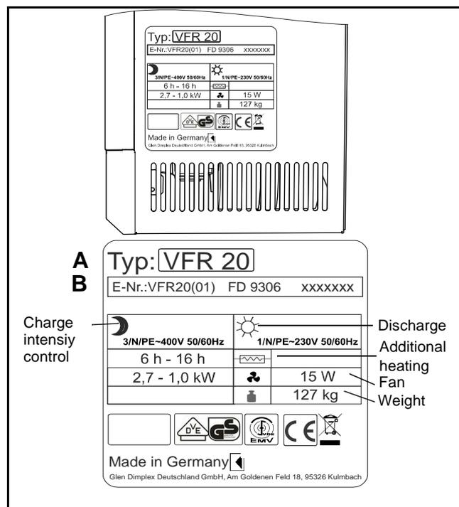
Fig. 25: Type plate on side panel
