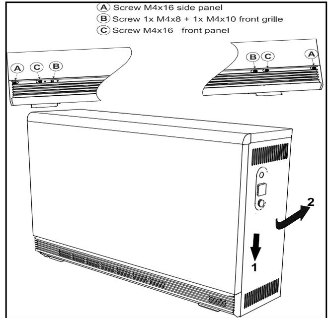
Fig. 8: Remove the screws from both side panels (A). Slide the side panels downwards (1) and swing them out (2). After the side panels have been removed, unscrew the fixing screws (B) on the front grille and remove the front grille. Then unscrew the fixing screws (C) for the front panel.
