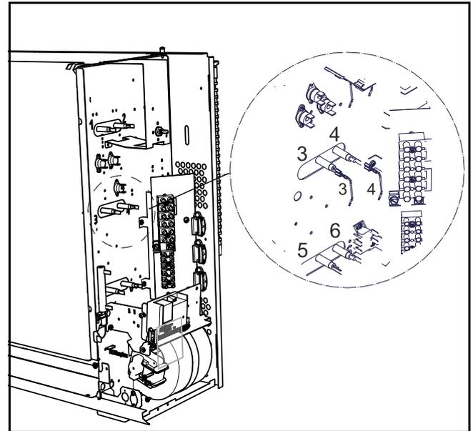
Fig. 20: The partition panel and the heating element supply cables are numbered (1 to 6). Connect the power supply cable wires to the storage heater connectors. Secure loose cables in the cable harness.
