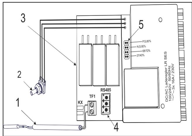
Fig. 24: Charge controller components
