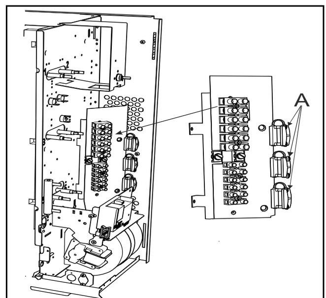
Fig. 21: Insert the electrical cables and make sure they are not subject to strain (A). Reduce the length of the cables so that they cannot come into contact with the heater's hot surfaces when it is operating. Do not allow the cables to lie in loops behind or underneath the storage heater!
